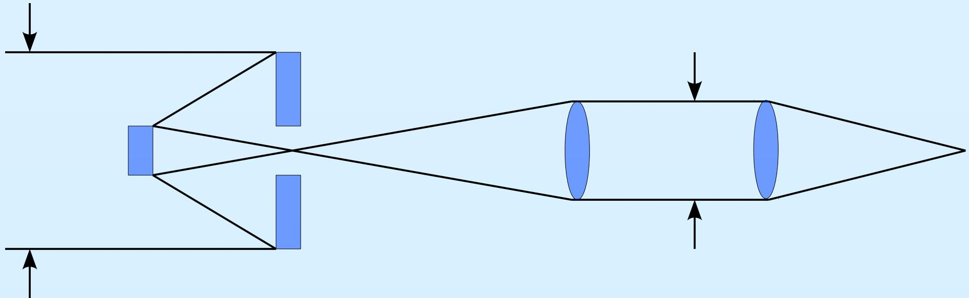
Ratio of diameters determines magnification
