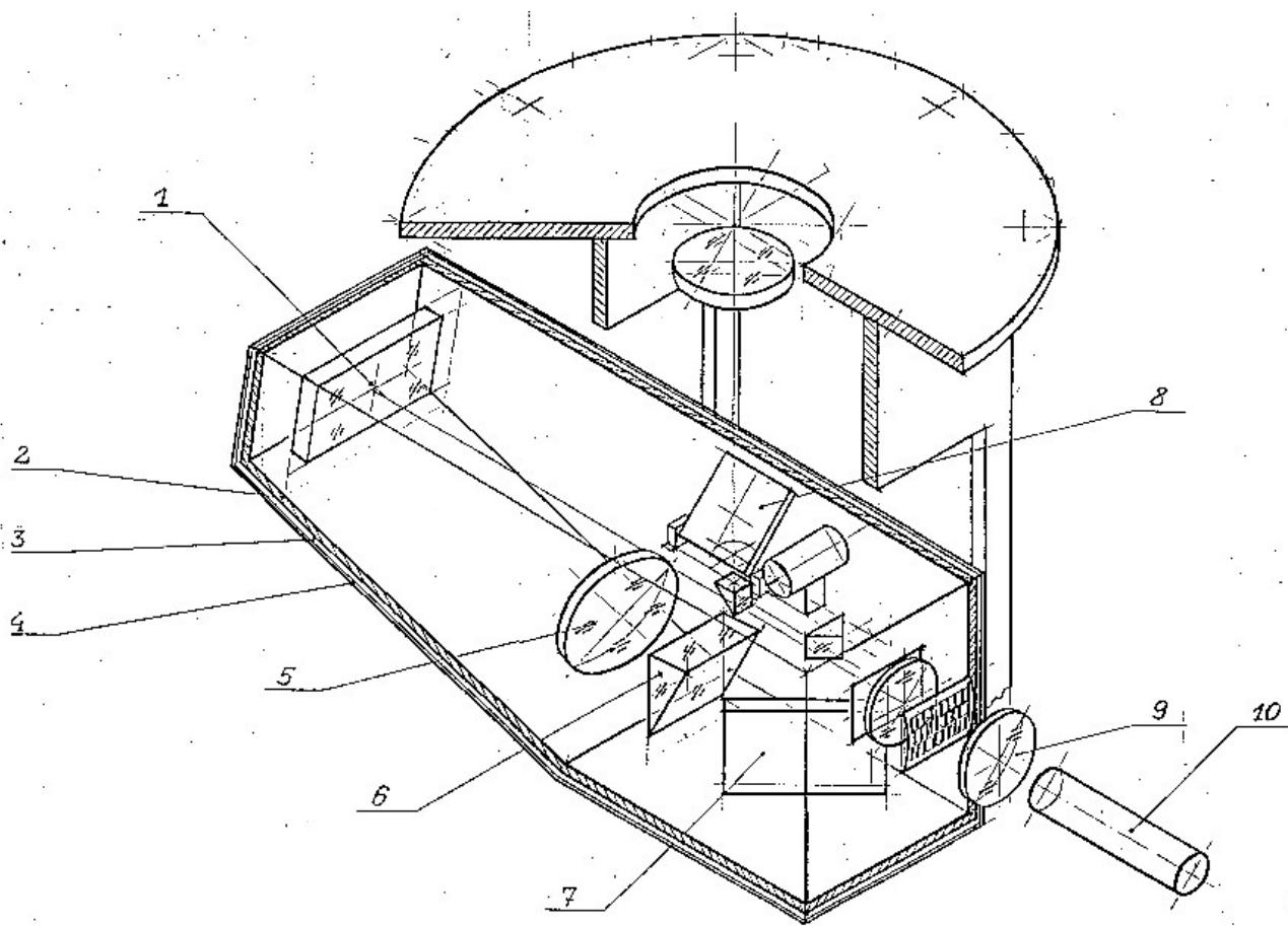
**Schematic diagram and principal components of the CORAVEL-type stellar radial-velocity spectrometer**
