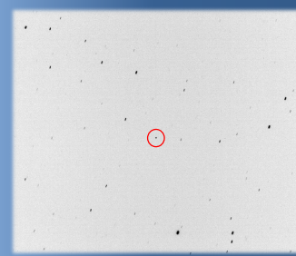
The Earth flyby of BepiColombo (circled point source) on 10/4/21. Our observations were combined with other data to simulate the trajectory of the spacecraft as a potential NEO threat (Micheli et al. 2021). The stars appear trailed.
